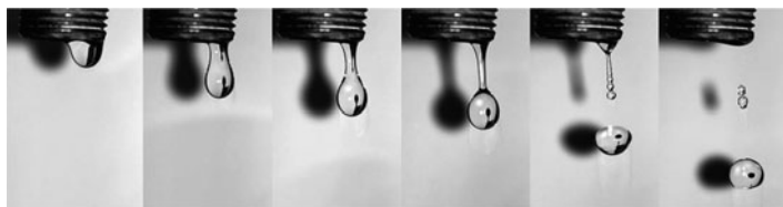
FIG 46 Sequence of changes of shape for a detaching droplet – practice.
